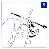
Take the old piece of tubing you saved and line it up with the newly threaded tube. Cut the end to the same length.
