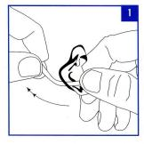
Pull the old tubing out of the earmould. Do not throw the old tubing away as you will need it later.
