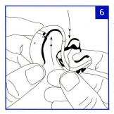
Push the end of the tubing onto the plastic nozzle on your hearing aid.
