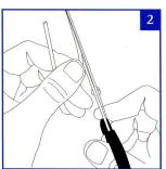
Cut the last 5cm (2 inches) of a pre-bent piece of tubing to a tapered end.
