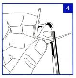
Cut the tapered tubing as close as possible to the earmould. Any tube sticking out could rub your ear and make it sore.
