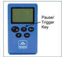
Trigger mode - you can manually trigger the machine to contract e.g. to practice picking things up.
