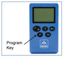
While the channel button is still flashing adjust the intensity level until you get the contraction you want. If it has stopped flashing before you are ready, press CH again.
