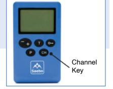
While channel (A or B) is flashing, select program by pressing P
